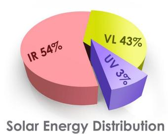
Solar properties for fenestration systems are calculated following recommended industry standard procedures. The recommended procedures and solar properties for the window film industry are stated in AIMCAL documents. The figure below shows the direct solar energy distribution. This shows the contribution to the SHG of each spectral region to any given glazing system.
